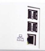
4 USB ports for data transmitting and connection with printer, keyboard, mouse, barcode scanner etc.
